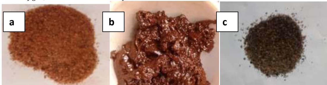
Fig. 1 (a) beach sand (b) mixture of glucose with sand (c) Final product GSC. The final product obtained as further milled in order to reduce its particle size
